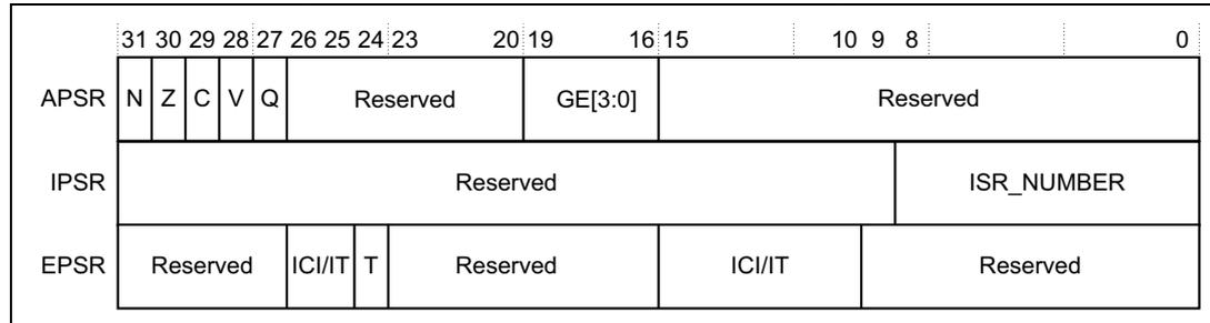
**Figure 4. PSR bit assignments**
